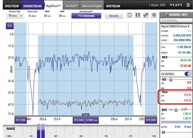
Figure 3. VSE-1100 measurement showing excessive digital hum; both the live and max hum results show the QAM degradation (as well as the live and min DQI results).
