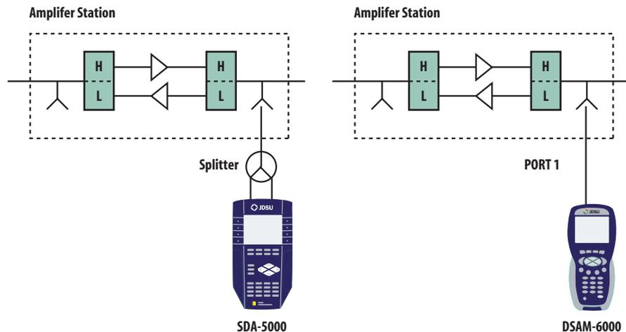
Systems with directional test points are preferred. A directional coupler is incorporated on the amplifier under test. Both the SDA and the DSAM are connected the same way. Two jumper cables are used, one for the forward sweep and another for reverse sweep.
