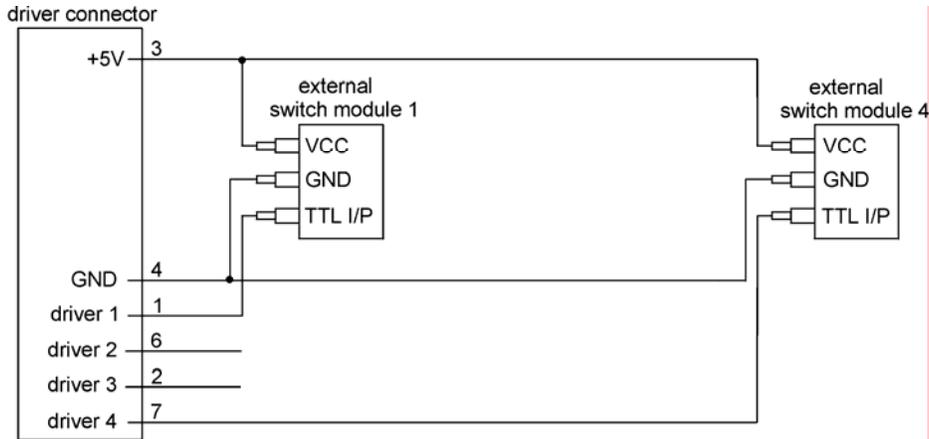
Figure 11: Switch Setup with TTL
