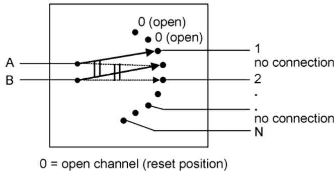
**Figure 5: Dual-Common Blocking Configuration**
