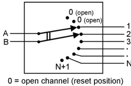
**Figure 4: Single-Step Dual-Common Configuration**
