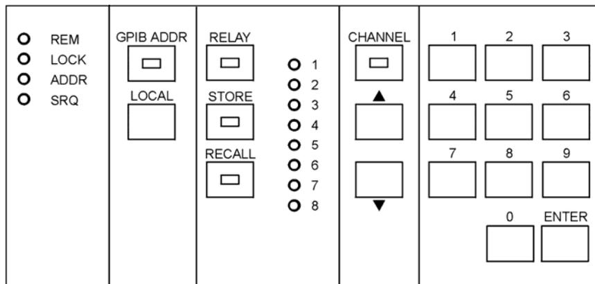
**Figure 8: Operating Keys and Status LEDs**
