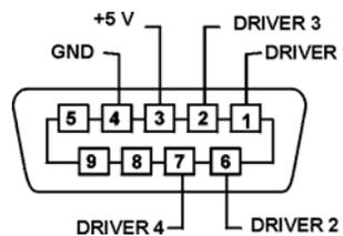
**Figure 17: RS232 Driver Pin Assignment**
