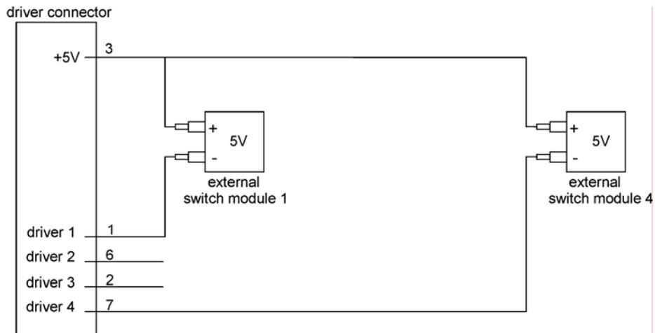
Figure 10: Switch Setup without TTL
