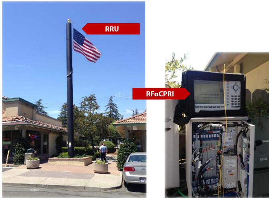
Figure 26. Small cell and CellAdvisor with RFoCPRI
