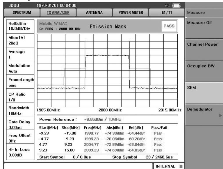
Figure 2-14 SEM measurement screen.
