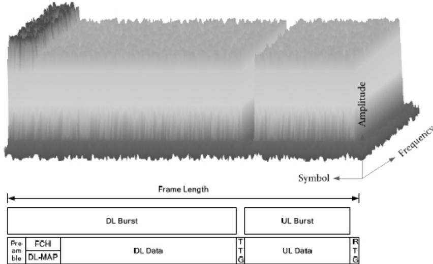
Figure 1-7 Frame structure of WiMAX signal using TDD
