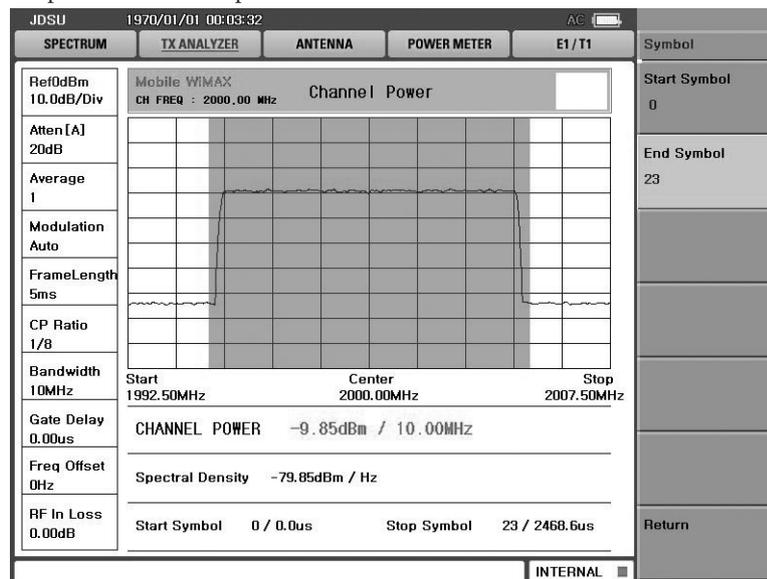
Figure 2-3 Channel Power Measurement screen
