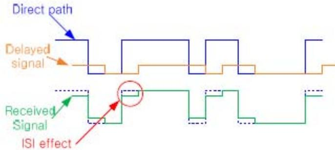
Figure 1-5 Distortion of received signal due to ISI
