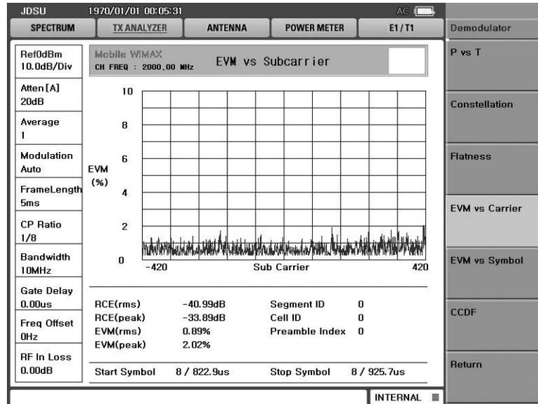
Figure 2-10 EVM vs. Sub-carrier Measurement screen
