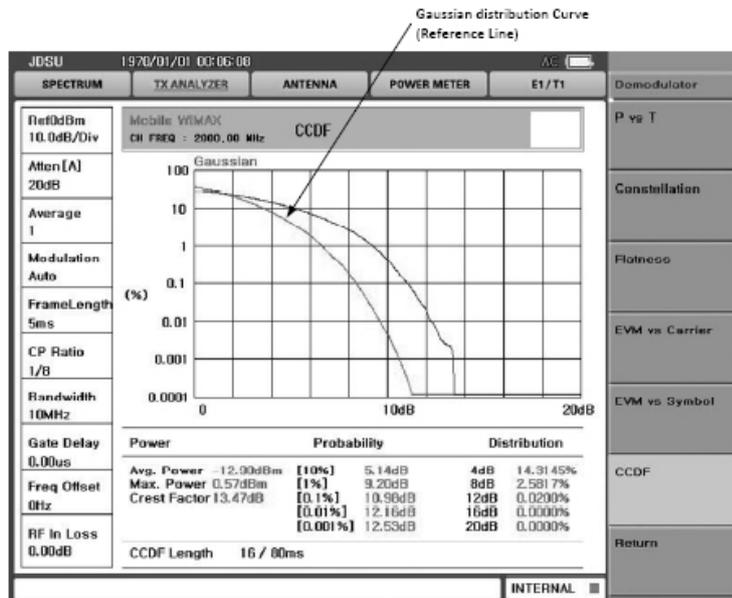
Figure 2-16 CCDF measurement screen
