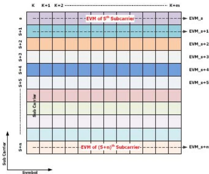
Figure 2-9 Frequency and time Interval setting scheme for EVM vs. Sub-carrier measurement
