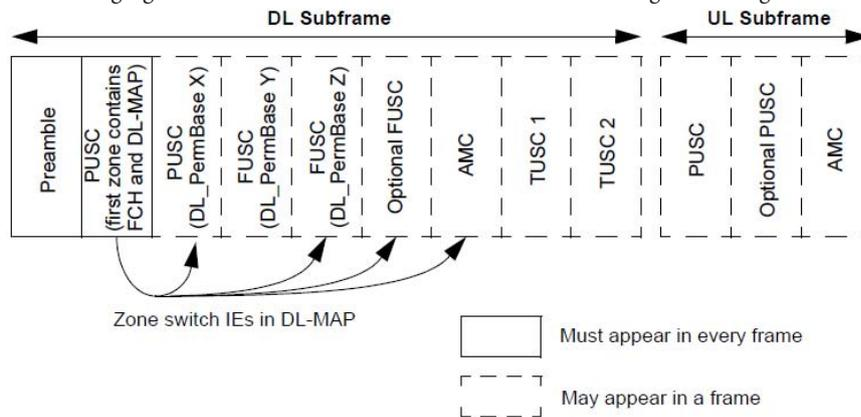
Figure 1-8 OFDMA frame consisted with multiple zones
