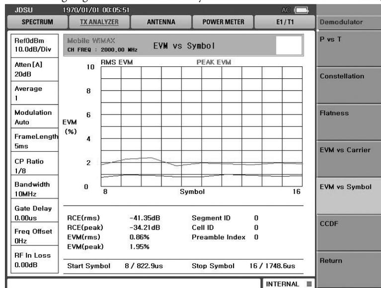
Figure 2-8 EVM vs. symbol measurement screen
