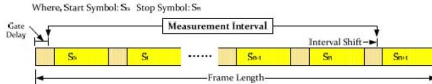
Figure 2-2 Gate delay setting
