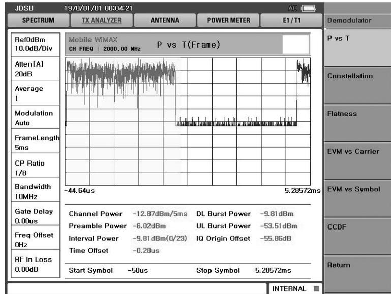
Figure 2-4 P vs. T measurement screen
