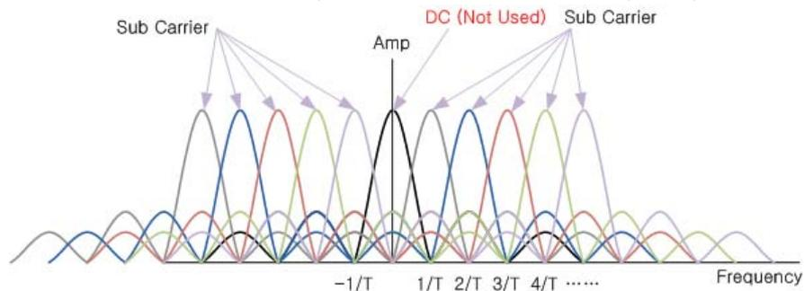
Figure 1-2 Sub-carrier allocation spacing vs. null periods
