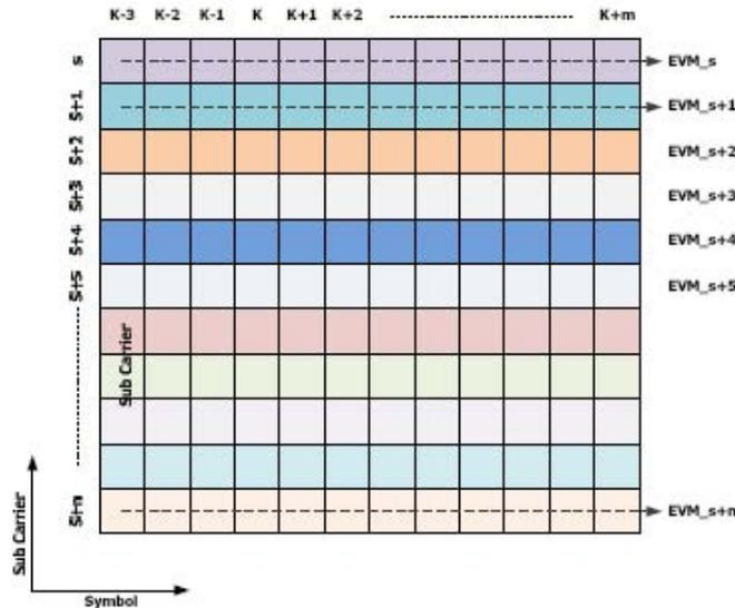
Figure 2-11 Sub-carrier selection scheme for RCE measurement
