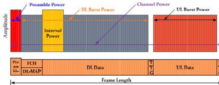
Figure 2-5 P vs. T measurement scheme
