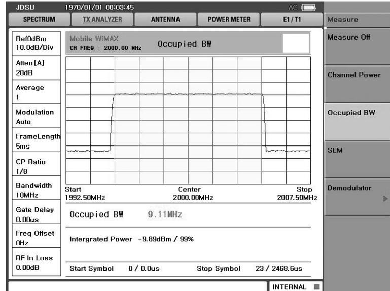
Figure 2-17 Occupied Bandwidth measurement screen
