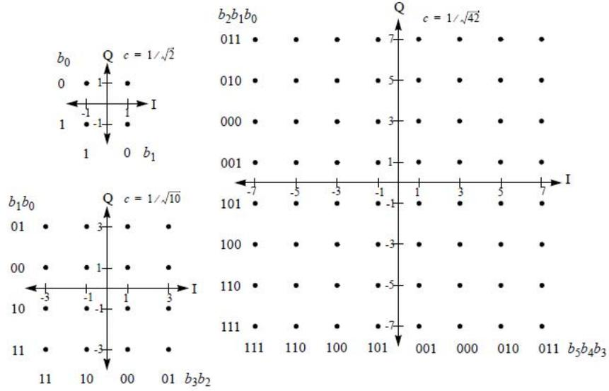
Figure 1-4 QPSK, 16QAM and 64-QAM constellations
