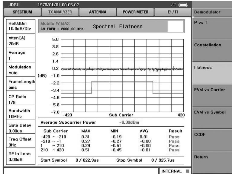
Figure 2-6 Spectral Flatness measurement screen
