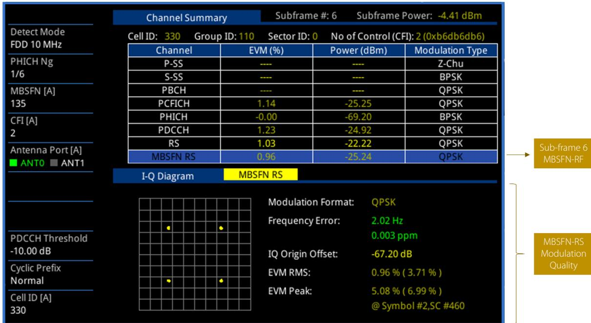
Figure 10. CellAdvisor MBMB SFN reference signal (MBSFN RS)
