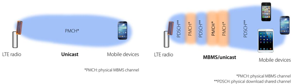
Figure 3. Unicast (PDSCH) and broadcast (PMCH) transmissions
