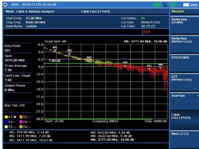
Cable and antenna test — Cable Loss
