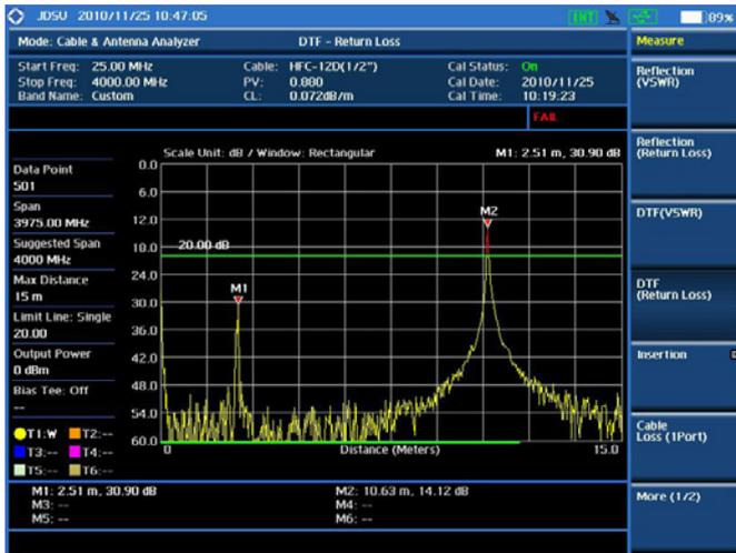
Cable and antenna test — Distance to Fault
