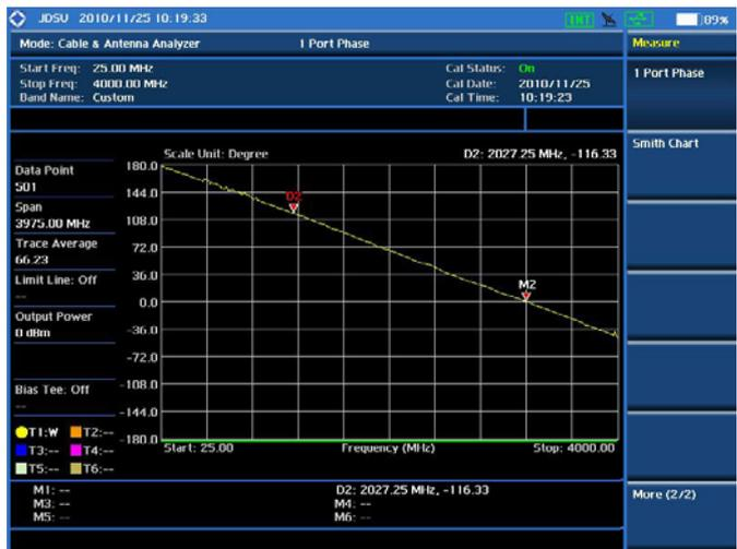
Cable and antenna test — 1-Port Phase
