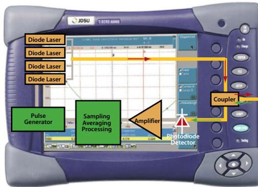
Figure 30: JDSU Pulse Delay OTDR method in the T-BERD/MTS-6000 platform
