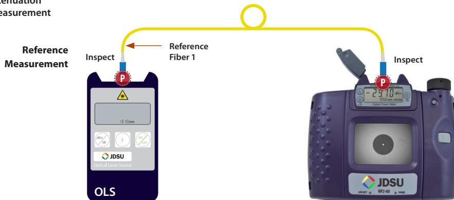
1. **INSPECT**, and if necessary, **CLEAN** both the ends of **reference fiber 1**.
