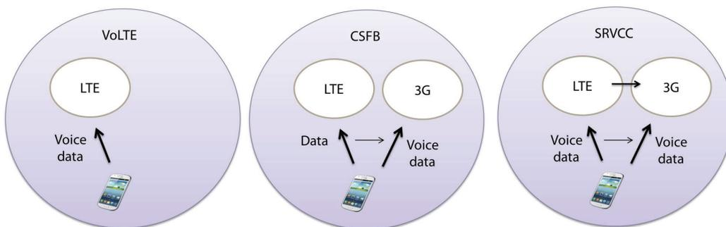
Figure 11. The span of VoLTE, CSFB, and SRVCC
