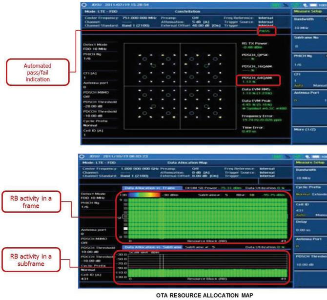
Figure 13. LTE RF signal analysis of VoLTE: demodulation and resource block analysis
