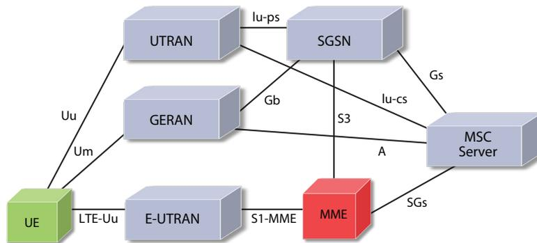
Figure 9. CSFB elements and interfaces (source: 3GPPTS 23.272 V10.14.0)
