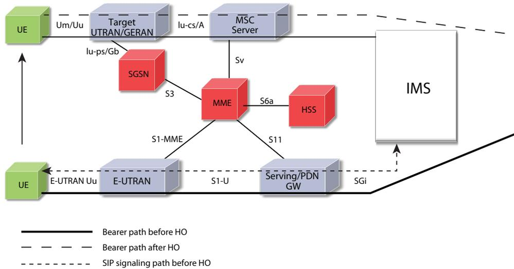
Figure 10. SRVCC elements and interfaces (3GPP TS 23.216 V10.6.0)
