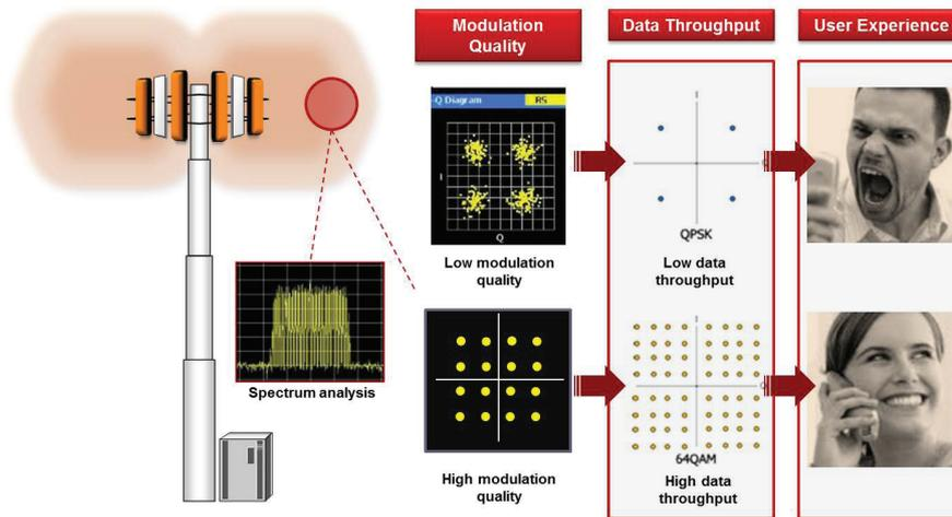
Figure 14. LTE signal analysis; LTE modulation quality indicates the modulation scheme and data throughput assigned to each user
