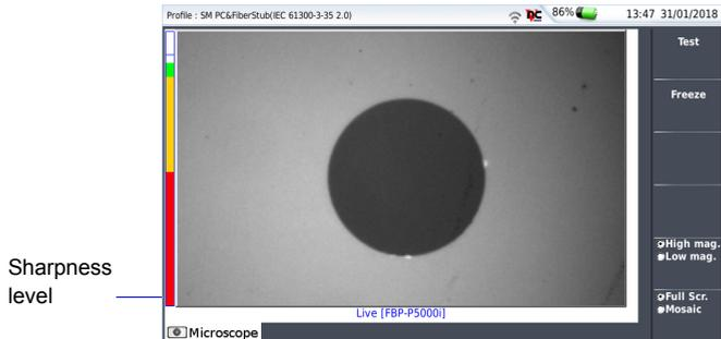
Use the **Focus Control** button onto the P5000i scope (see [Figure 21 on page 50](#)) to adjust the image quality and sharpness.
