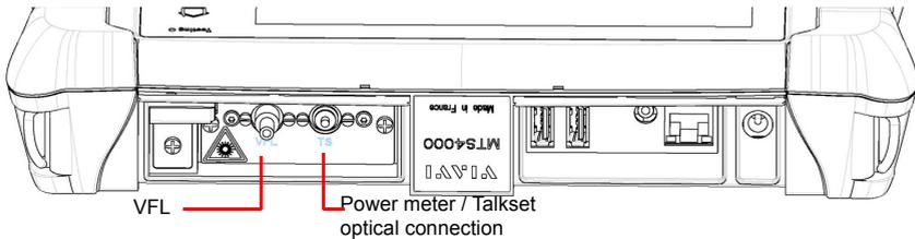
The type of optical connector used for the power meter is UPP (Universal Push Pull), which is compatible with all diameter 2.5 mm connectors (FC, SC, ST, DIN, E2000, etc.)
