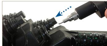
2. Insert the CleanBlast system into the OptiTap receptacle.
