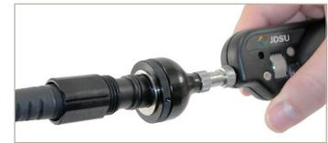
3. Align the **arc and flat** geometry of the OptiTap 2.5 mm APC plug connector to the matching "female" counterpart insertions on the probe tip/adapter and insert/attach. Adjust focus and inspect the plug.
