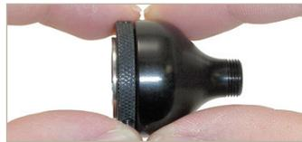
1. Align the inspection adapter to the flare adapter and attach. Screw in to tighten and secure.
