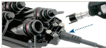
2. Align the **arc and flat** "male" pin geometry of the inspection tip to the matching "female" counterpart insertions inside the OptiTap receptacle adapter and insert to secure.
