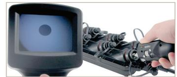
3. Apply light pressure to get optimal contact with the fiber end face, adjust focus and inspect.
