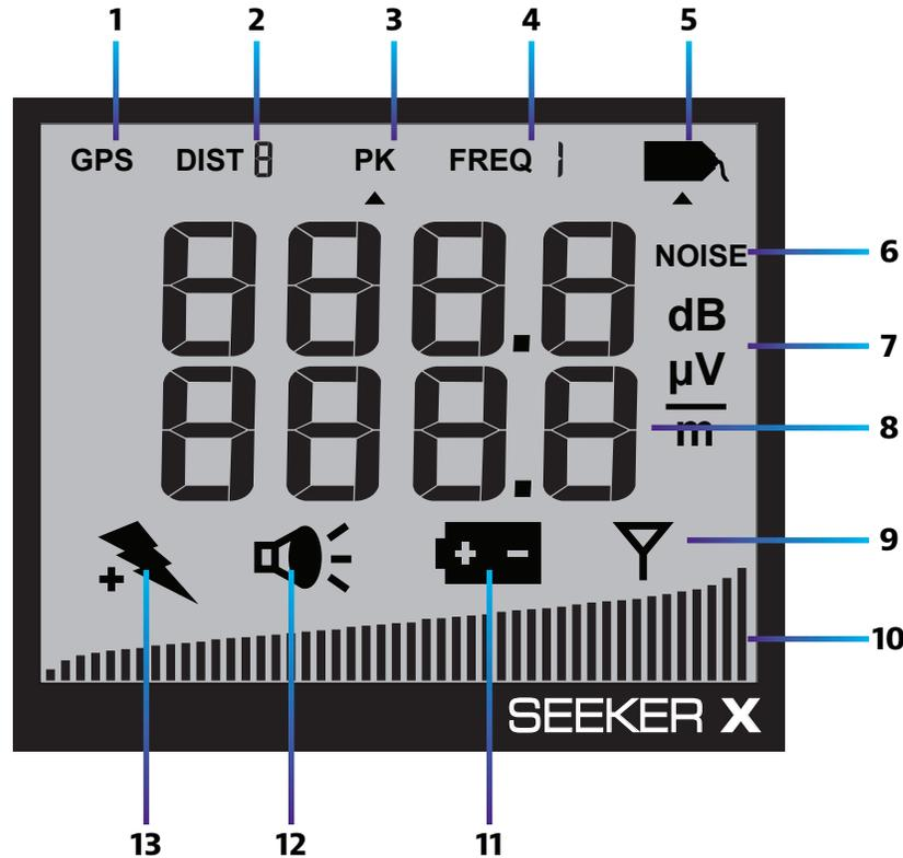
1. **GPS** – Shown when the meter is placed in the Mobile Mount and a GPS connection is established with an optional Seeker MCA III. When the icon is not shown, the meter is not in the Mobile Mount or the GPS connection cannot be established with the optional Seeker MCA III. If the icon flashes, the Seeker MCA III is connected to the GPS but the GPS does not have a good position fix.
