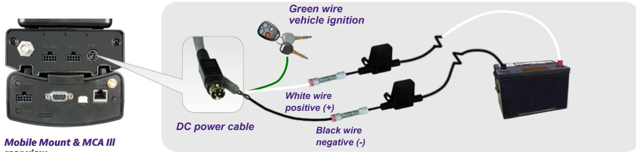
*\*Use the provided in-line fuse holders to wire the white & black DC power cables to the vehicle battery as shown. Wire the green DC power cable to the vehicle key switch to allow the MCA III to determine when the vehicle is turned OFF.*
