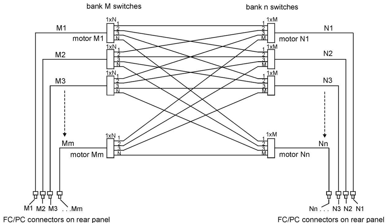
Figure 2: General Schematic of an SG MxN Switch
