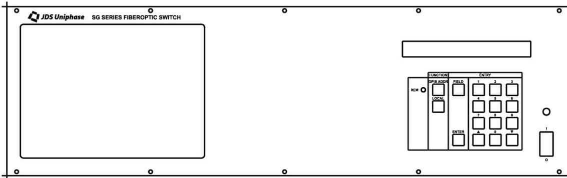
Figure 5: Front Panel of 3USG with keypad
