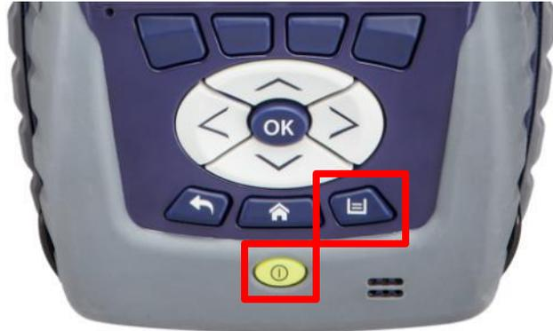
Hold UTILITY KEY simultaneously during POWER button press. Continue to hold UTILITY KEY until LEDs flash ORANGE, then release UTILITY KEY
