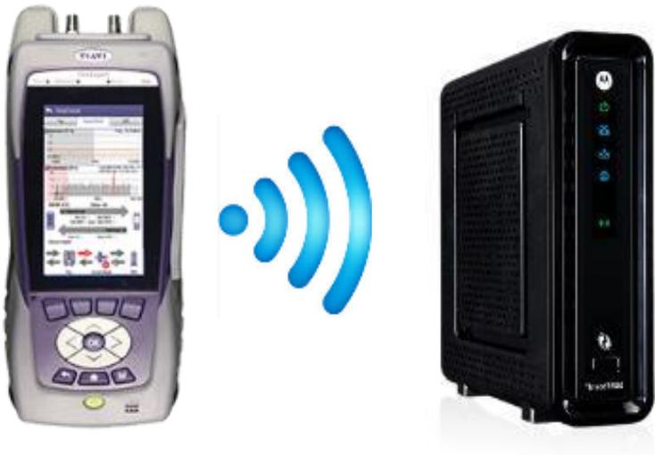
From the ONX home screen navigate to **SYSTEM NETWORK / WIFI** - Verify the ONX has a valid IP address
