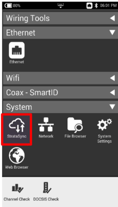
After IP Address verification, navigate to the **SYSTEM** Menu and select **STRATASYNC**
