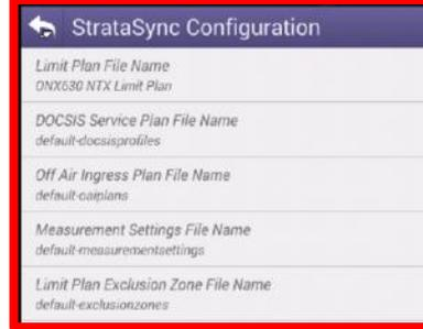
User can verify that configurations are correct and up to date by selecting VIEW STRASYNK CONFIGURATION
