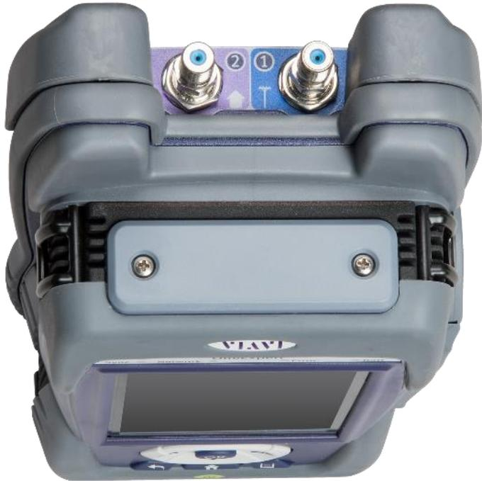
The ONX-CATV has two RF ports with field replaceable barrel style connectors. The ONX ships with two F- 81 splice style adapters rated to 3 GHz. These F-81 adapters are 1.2 in (307mm) long with a 0.5 in (132mm) distance between either end and the tightening nut. They are shipped installed into the RF ports to the recommended torque specification of 20 in-lbs. (1.6 ft-lbs.).
