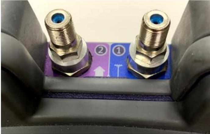
Start by removing the current F-81 adapter and collar (if present). If needed use a 7/16 wrench, turn the F connector counterclockwise until the adapter is completely out of the ONX RF port. Retain the collars if not replacing them with new ones.
