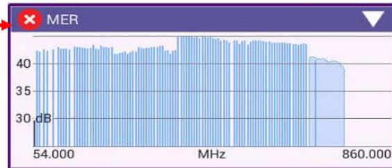
MER shows the value of all the QAM channels in the system in a bar graph
