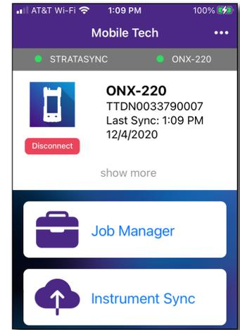
To obtain the latest configuration settings, software options and updates, and ownership registration information, the OneExpert can sync with a VIAVI server via the internet. The synchronization also stores any user files saved on the unit to the StrataSync server.
