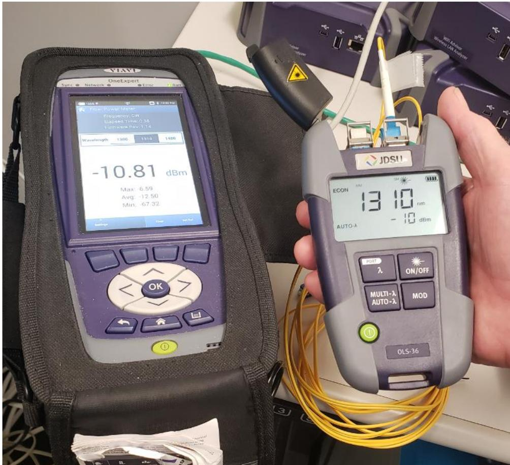
In this picture an optical light source (OLS-36) was used to transmit -10 dBm in the 1310 nm Wavelength, and then -10.81 dBm is being read by the Power Meter and displayed in the OneExpert CATV meter screen. Thus, a loss of 0.81 dBm is observed.
