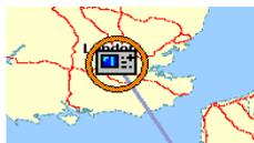
The RTUs in alarm are circled, the color representing the severity of the alarm detected.
