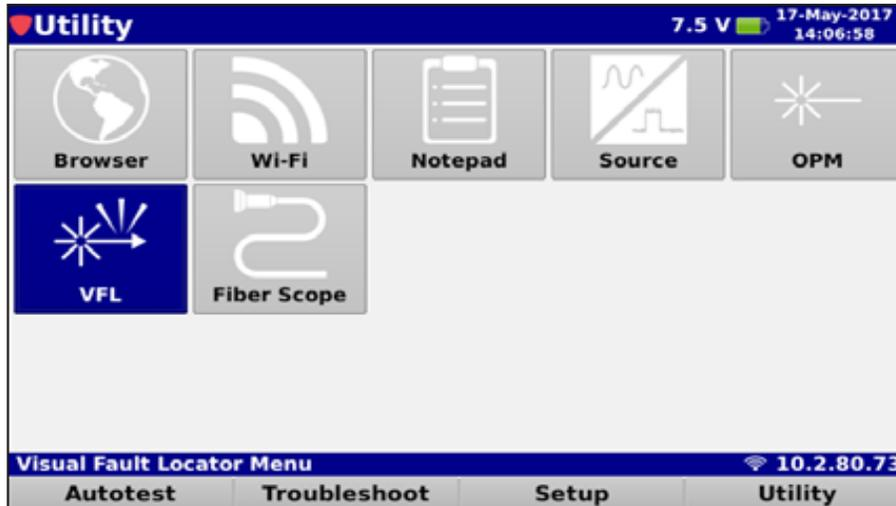
The VFL meter will be displayed as shown here. The Laser Power is off by default.
