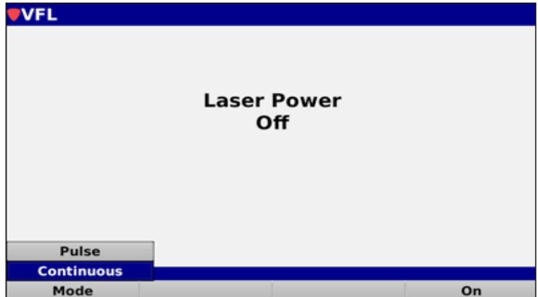
Select the **On** softkey to activate the laser power to the VFL. After selecting the On softkey, the screen shown in the image to the right is displayed for two seconds before activating the laser output.
