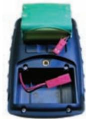
1. Unscrew the hex screw on the battery compartment with the hex key (included).
