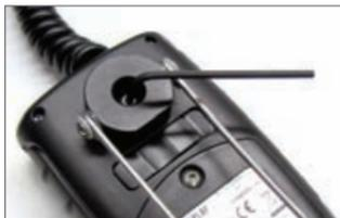
*Use the hex tool to tighten the hex screw on the accessory and secure onto the back of the HD3 display.*
