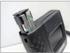
1. Insert 8 "AA" batteries into the battery pack.
