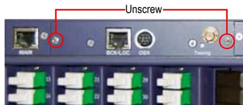
Fig. 25 GSM option on front panel
