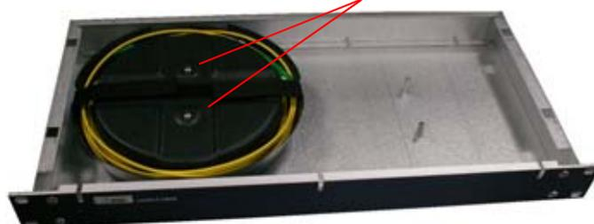
Fig. 36 Installation of the Fiber Launch
