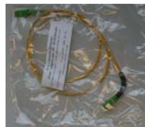
Angled Jumper with the correct connector
