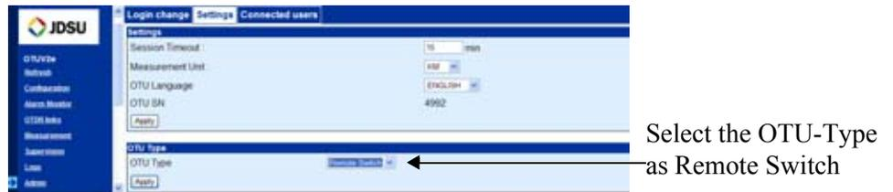
**Fig. 53** Remote Optical switch configured
