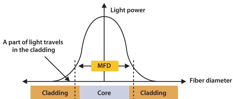
Singlemode fiber has a larger mode field diameter at 1550 nm than at 1310 nm and at 1625 nm than at 1550 nm. Larger mode fields are less sensitive to lateral offset during splicing, but they are more sensitive to losses incurred by bends during installation or in the cabling process.
