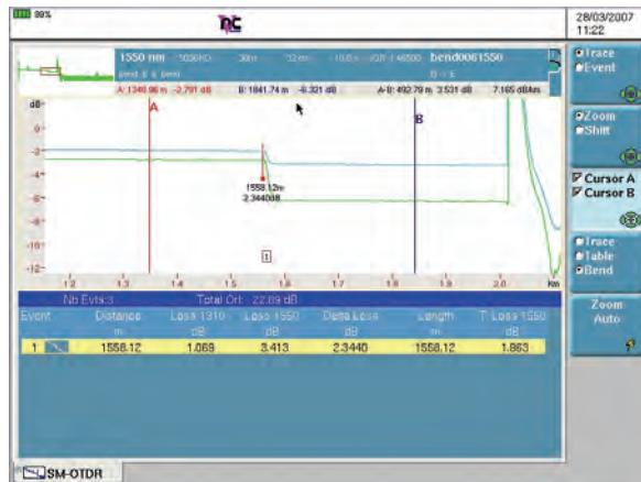
Bend analysis between 1310 and 1550 nm with the T-BERD/MTS 6000
