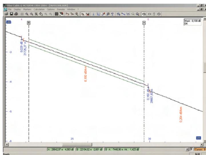
Using the mask function of JDSU OFS-100 for fiber tension analysis
