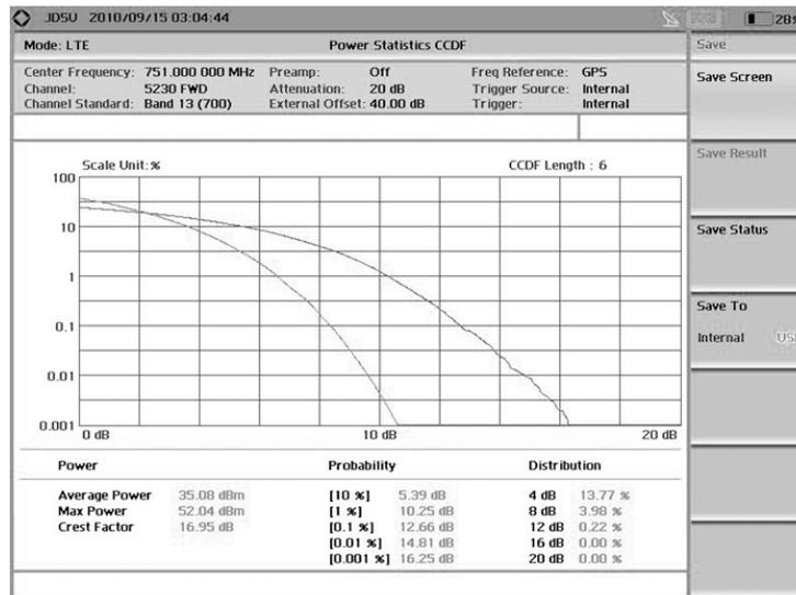
Figure 19. CCDF measurement for TM1.1
