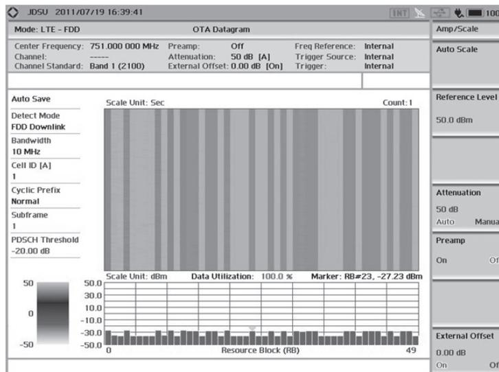
Figure 35. Over-the-Air Datagram Measurement
