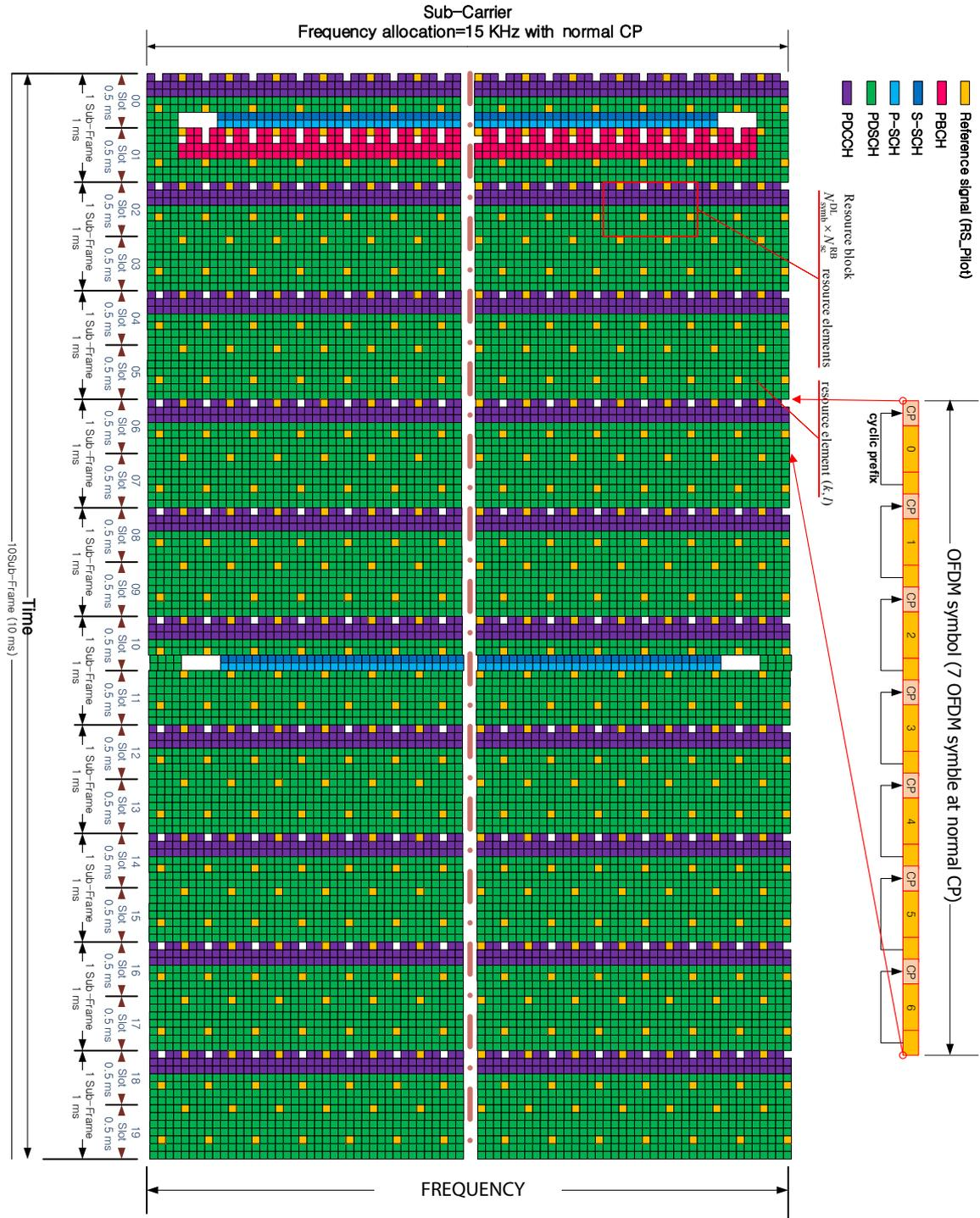
Figure 16. Downlink map of 10 ms LTE frame ( $\Delta f=15$  KHz, normal CP)
