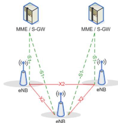
Figure 1. LTE Overall Architecture <sup>(Ref. 2)</sup>
