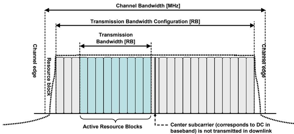
Figure 3. LTE channel bandwidth and transmission bandwidth (Ref. 3)
