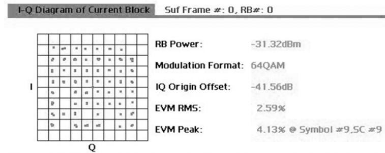
Figure 27. I-Q diagram in the Subframe Summary measurement
