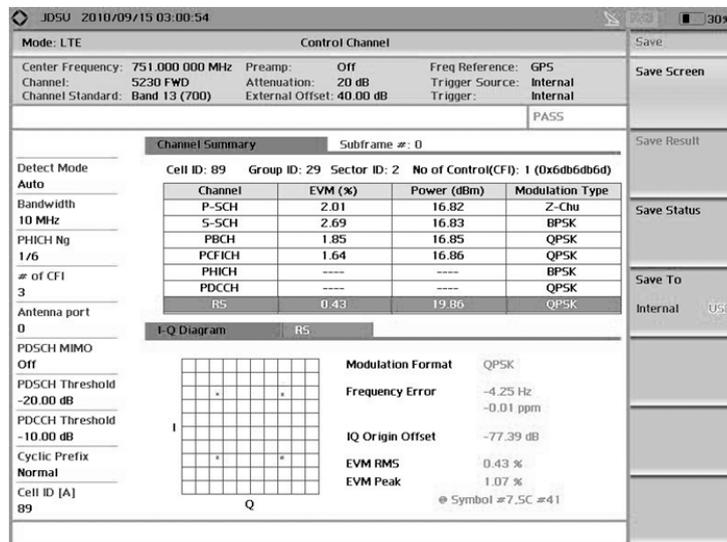
Figure 28. Control Channel Summary measurements
