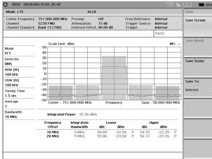
Figure 31. ACLR measurement screen (E-TM1.2)
