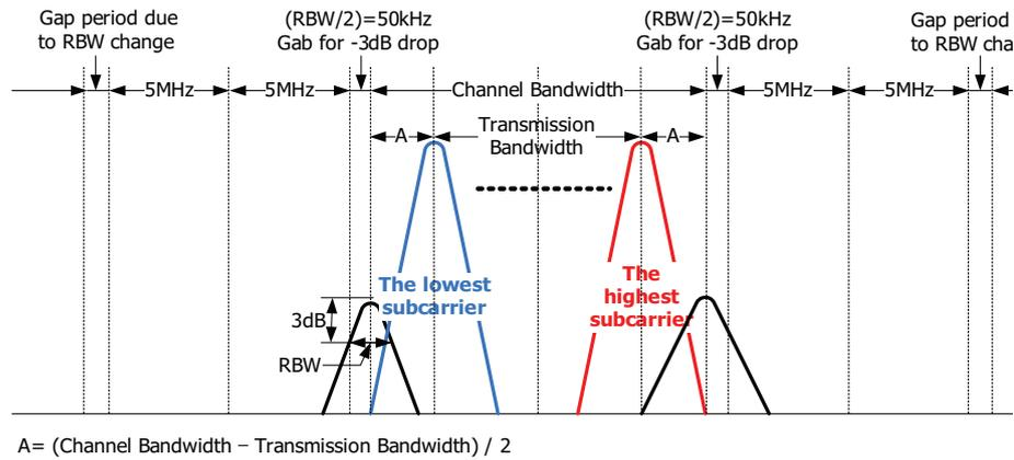
Figure 32. Definition of SEM sections
