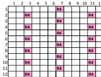
Figure 13. Mapping of MBSFN RSs (extended cyclic prefix  $\Delta f = 15$  KHz) <sup>(Ref. 1)</sup>
