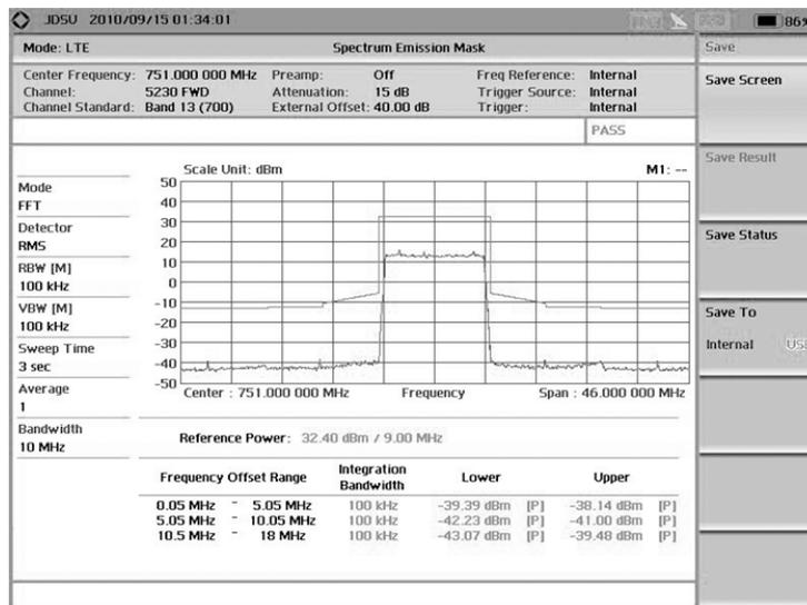
Figure 33. SEM measurement (E-TM1.1)
