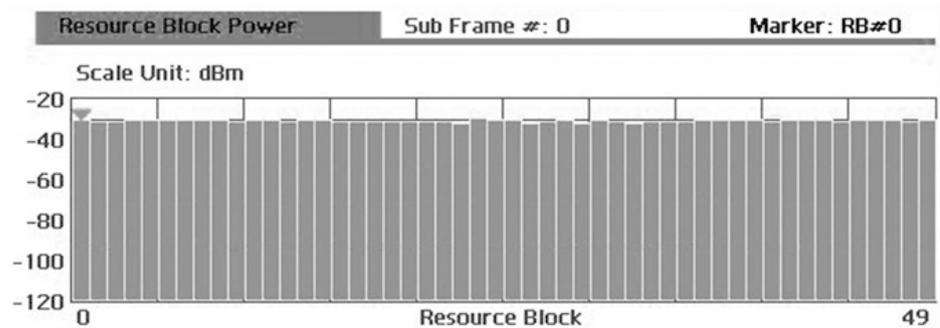
Figure 26. Resource block power diagram in Subframe Summary measurement
