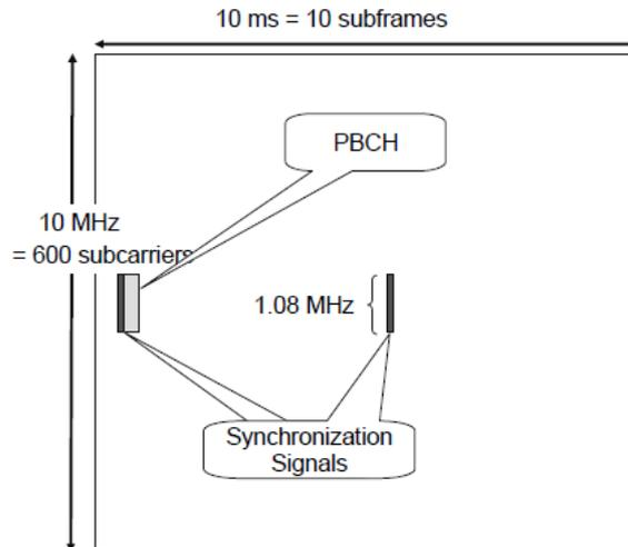
Figure 11. PBCH location at the center frequency
