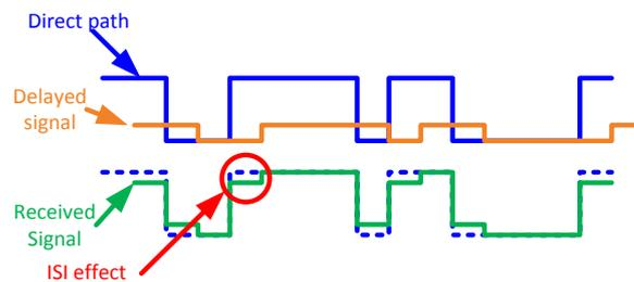
Figure 6. Distortion of received signal due to ISI
