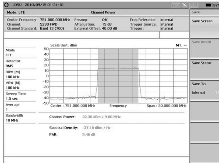
Figure 17. Channel power measurement (E-TM1.1)
