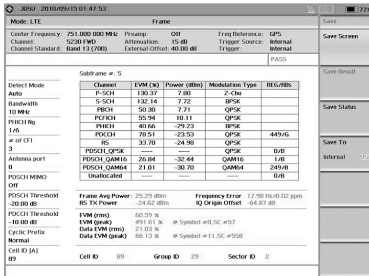
Figure 20. Frame Summary measurement for 10 MHz LTE DL signal (E-UTRA TM3.2)
