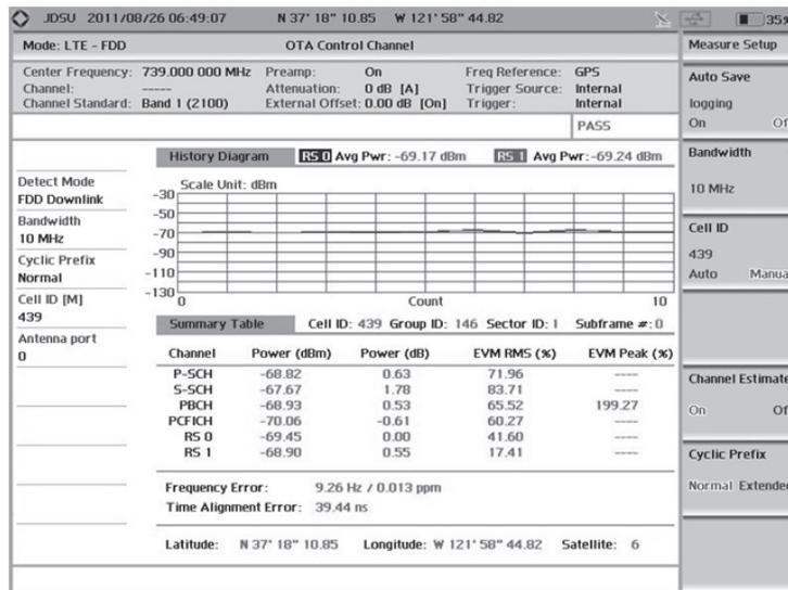
Figure 36. Over-the-Air Control Channel Measurement
