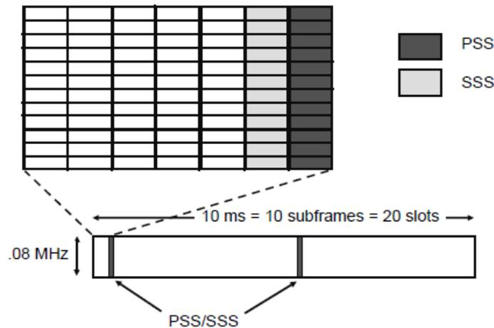
Figure 15. Synchronization signals in the frame
