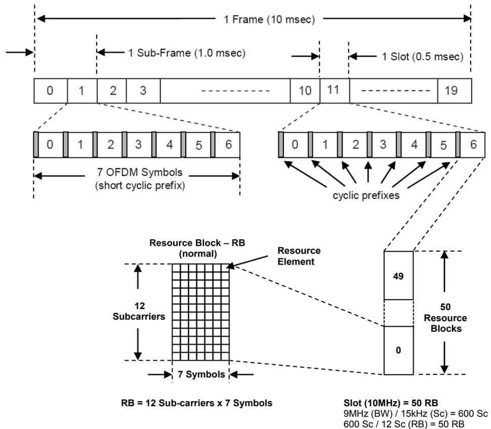
Figure 4. LTE frame structure
