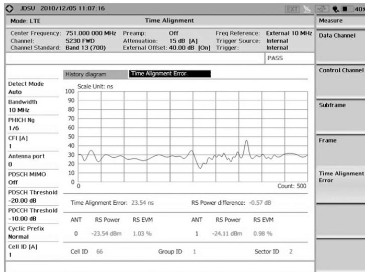
Figure 29. MIMO Time Alignment measurement
