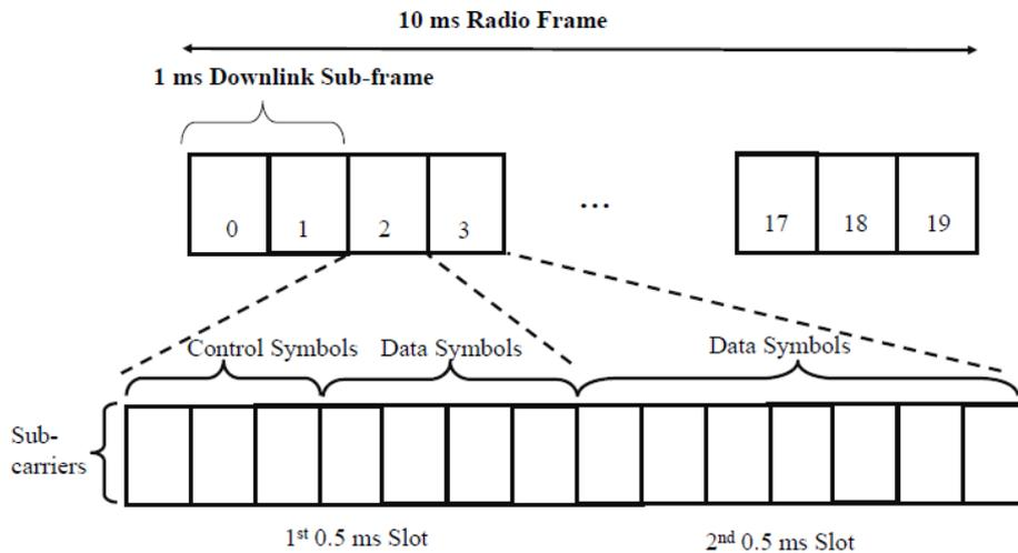
Figure 9. Downlink slot structure for bandwidth above 1.4 MHz
