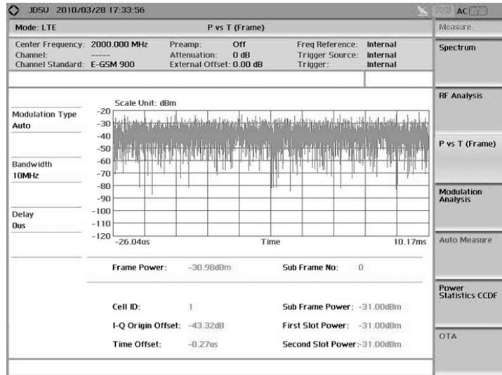
Figure 18. Power vs. Time measurement for TM1.1
