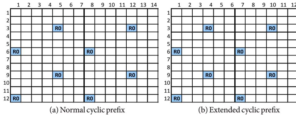
Figure 12. Mapping of downlink RSs for SISO <sup>(Ref. 1)</sup>
