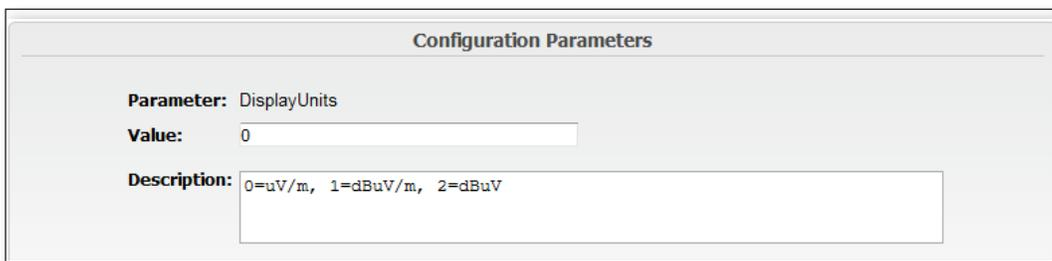
The screenshot shows a configuration window titled "Configuration Parameters". It contains three fields: "Parameter" with the value "DisplayUnits", "Value" with the number "0" entered in a text box, and "Description" with the text "0=uV/m, 1=dBuV/m, 2=dBuV" entered in a larger text box.
