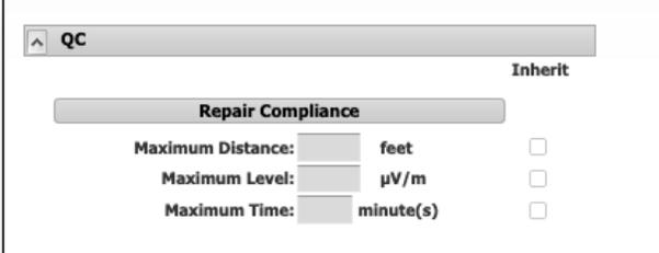
The screenshot shows a software window titled "QC" with a sub-section "Repair Compliance". It contains three rows of settings, each with a text input field, a unit label, and an "Inherit" checkbox. The first row is "Maximum Distance: [input] feet" with an unchecked checkbox. The second row is "Maximum Level: [input] µV/m" with an unchecked checkbox. The third row is "Maximum Time: [input] minute(s)" with an unchecked checkbox. The "Inherit" label is positioned to the right of the top row.
