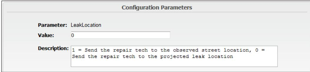
The screenshot shows a window titled "Configuration Parameters". Inside, there are three fields: "Parameter:" with the value "LeakLocation", "Value:" with a text input field containing "0", and "Description:" with a text area containing the text "1 = Send the repair tech to the observed street location, 0 = Send the repair tech to the projected leak location".
