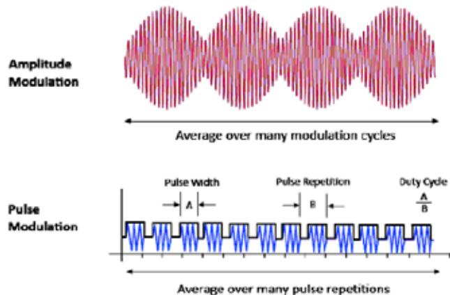
To measure average power accurately, the time constant of the sensing device must be sufficiently long with respect to the lowest frequency component in the signal being measured. The power of a modulated amplitude signal must be averaged over several cycles. Similarly, the power of the pulsed signal must be averaged over many pulse repetitions to obtain an accurate measurement. Test equipment for average power measurements is economical, easy to use, and most importantly accurate.
