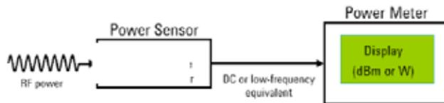
This above diagram shows the basic methodology of measuring high frequency power using the combination of power meter and power sensor. The power sensor converts high frequency power to a DC or low frequency signal that the power measure can measure and relate to an RF power level. The meter displays the direct signal as a power value in dB or watts.
