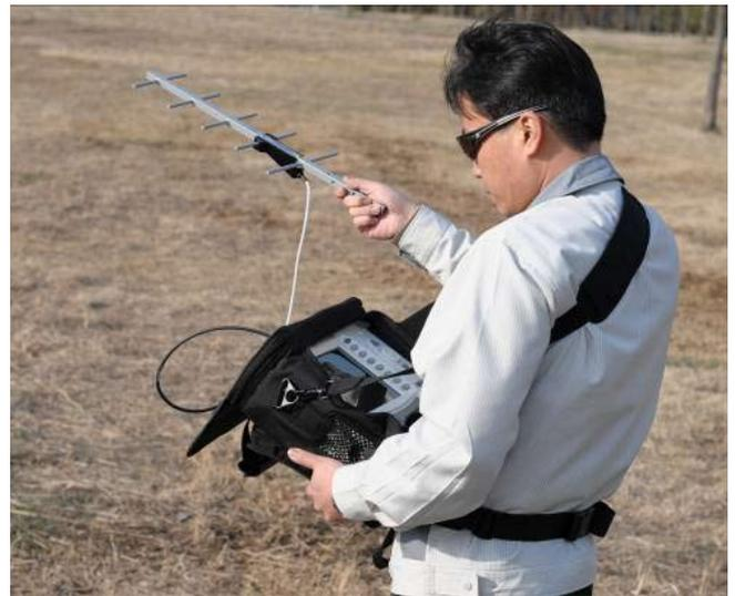
The **audible tone** is proportional to the signal power strength. In addition a built-in AM/FM audio demodulator it provides a convenient identification of AM/FM signals.
