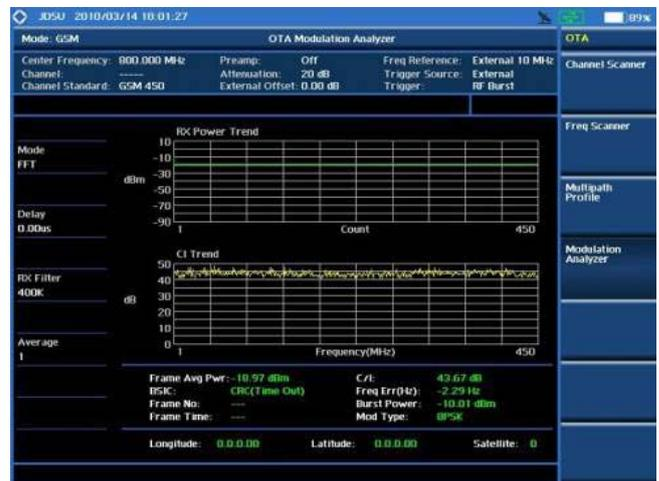
GSM OTA Modulation Analyzer
