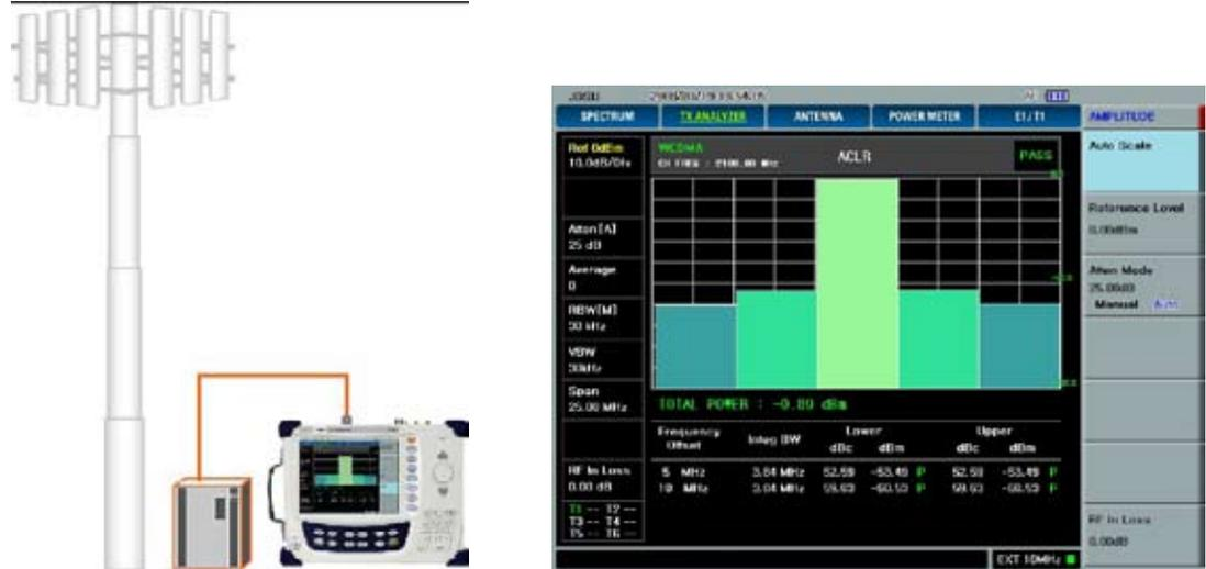
JD7105A WCDMA Adjacent Channel Leakage Ratio Measurement
