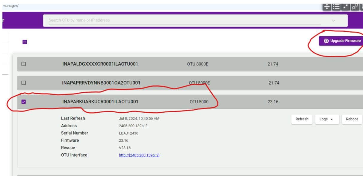
**2. Select Firmware to be upgraded and Part to be upgraded and press OK.**
