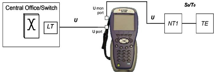
**Figure 8** Connecting as a U Monitor
