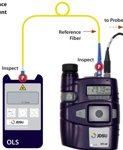
1. **INSPECT**, and if necessary, **CLEAN** both the ends of the **reference fiber**.
