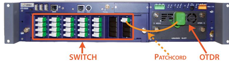
The patchcord between the OTDR and the SWITCH is supplied with the OTU-8000.
