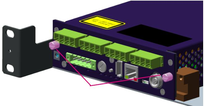
**4** Fix the whole assembly to the rack using the tools included into the E9E-RACK-MOUNT Kit.
