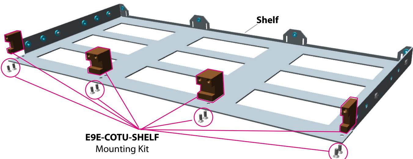
**2** Fix the brackets on both sides of the shelf, using the 4 screws M4x8, included into the RACK-LOCK-SCREW Kit.
