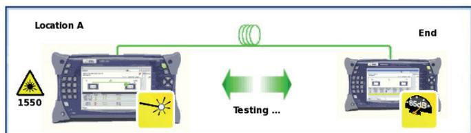
The test sequence can be initiated from one or the other unit. No additional intervention is necessary until the end of the measurement cycle. At the end of the test, all results are available at the same time.
