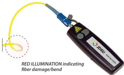
RED ILLUMINATION indicating fiber damage/bend
