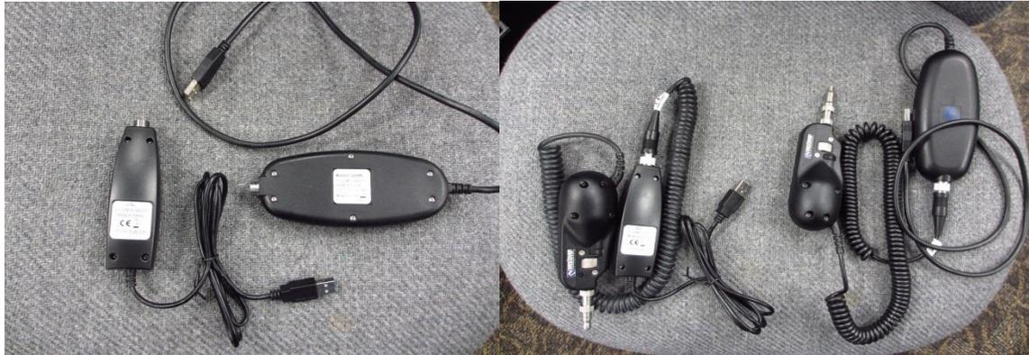
**OS Compatibility:** WIN2k, WIN XP, Win Vista (32 bit only). The main thing to remember about the analog probes is that they are NOT 64 bit OS compatible. A PC with WIN 7 running in 64 bit mode will not recognize the probe. The issue is not the FC2 or FC Pro software but rather the hardware in the USB converter.
