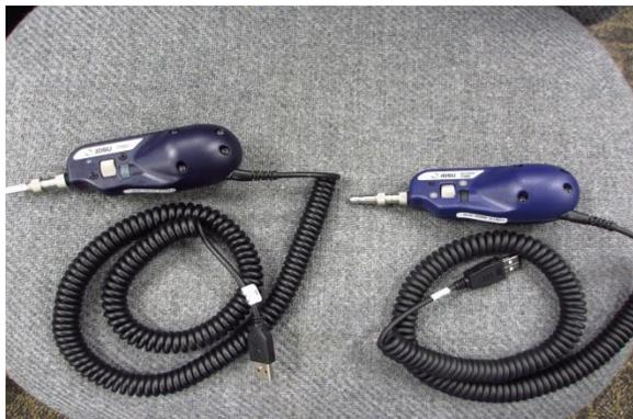
The probes look identical. They will be marked as a P5000i or P5000 (JDSU label on the side of the probe). You can also tell by the serial number marked on the bottom of the probe body whether the probe is a P5000 or P5000i.
