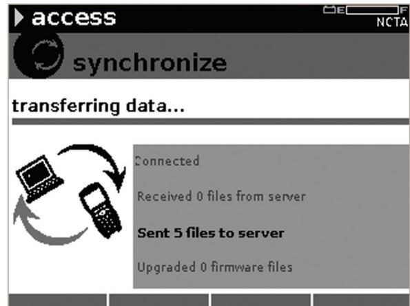
Users can synchronize test files from the field and administrators can update channel plans over Ethernet or DOCSIS RF connections.
