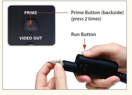
3. Attach the patch cord to the handset, push the connector into the handset to disengage safety mechanism (*the POWER/READY light will turn green*), and press the **run button** to initiate cleaning (*cleaning takes <1 second*).
