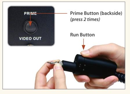
3. Insert the handset into the bulkhead and push to disengage safety mechanism (*the POWER/READY light will turn green*), and press the **run button** to initiate cleaning (*cleaning takes <1 second*).
