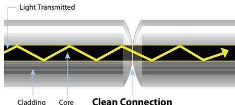
Today's connector design and production techniques have eliminated most of the challenges to achieving **core alignment** and **physical contact**.
