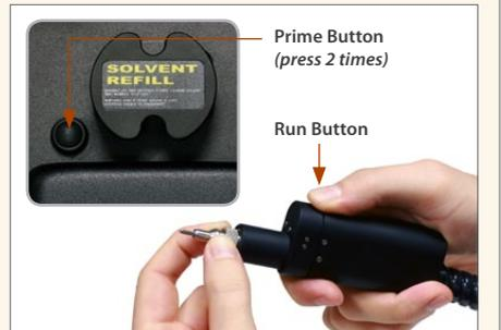
2. Attach the patch cord to the handset, push the connector into the handset to disengage safety mechanism (*the POWER/READY light will turn green*), and press the **run button** to initiate cleaning.
