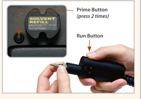
2. Insert the handset into the bulkhead and push to disengage safety mechanism (*the POWER/READY light will turn green*), and press the **run button** to initiate cleaning.
