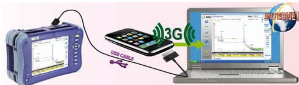
Fig. 60 Connexion USB via Smartphone 3G
