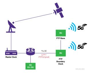
This scenario still uses the ITU-T G.8275.1 and SyncE profiles as previously described. The test points include any 10GE or 25GE interfaces on the DUs and RUs as well as any fronthaul transport network multiplexors and xWDM equipment to which the DU and RU may connect. Particular attention should be placed on testing Sync PDV at boundary clock locations to characterize filtering performance.
