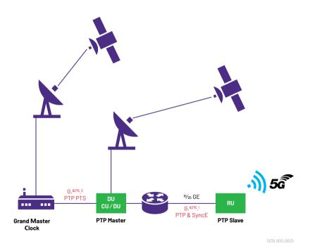
Similar to the APTS approach already mentioned, the PTS measurement methodology applies a low-pass filter to the selected packets. The pass/fail criteria are expressed in terms of taking the filtered packets and measuring that the absolute max |TE| over the lifetime of the measurement to ensure it does not exceed 1,100 ns. A 200 second window is still used and 0.25% of samples are taken in either direction between the grand master and the local master clock.
