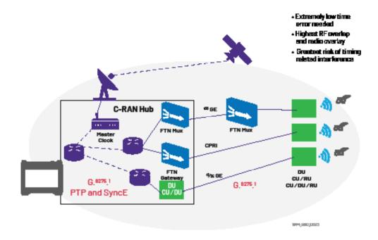
Large mobile networks require aggregation points to run efficiently. This is seen most often in large cities where population density requires increased coverage. In these types of situations, the focus is on supporting very tight synchronization requirements via tight boundary clock specifications within the area of coverage where the radios overlap the most. Synchronization with the rest of the network is relaxed but still complies with maintaining a Class 4 Network endto-end.
