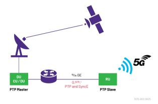
This scenario will also use the ITU-T G.8275.1 and SyncE profiles as previously described in the fronthaul aggregation application. The test points include any 10GE or 25GE interfaces on the DUs and RUs as well as any fronthaul transport network multiplexors and xWDM equipment to which the DU and RU may connect.
