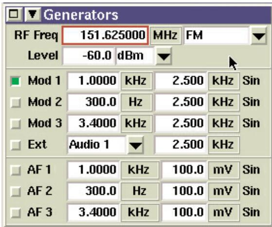
Figure 7.0 Proper Configuration of the 3901 Generator
