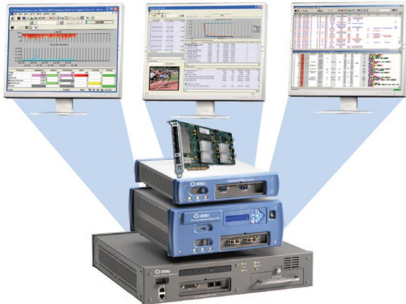
Distributed Network Analyzers and the 10 Gigabit/Gigabit Ethernet Interface card
