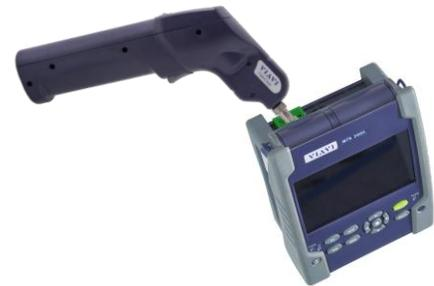
Figure 3: OTDR Port Inspection
