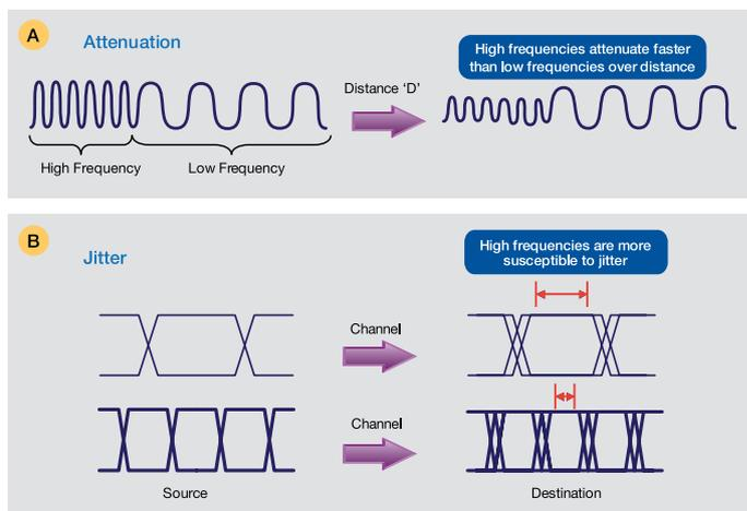
Gb/s SAS/SATA signals have increased sensitivity to attenuation and jitter. Higher frequencies attenuate faster than low frequencies over distance (A) and are more susceptible to jitter (B). Proper test setups reduce the additional attenuation or jitter introduced into a system during testing.
