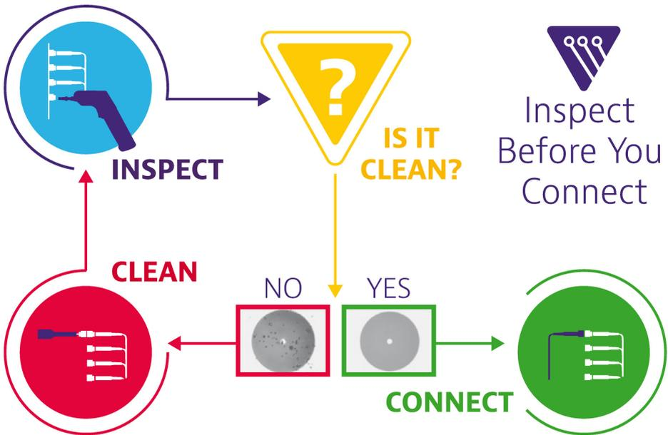
Never force the connector ferrule or insert it with an angle into the test port adapter. Mechanical stress may permanently damage the ceramic sleeve of the adapter or the end face of the connector.
