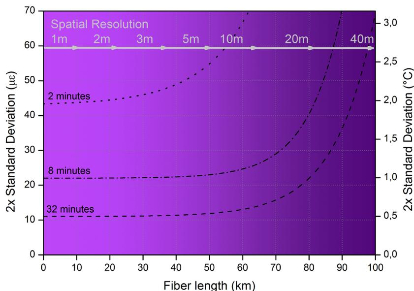
This is a repeatability chart with repeatability defined as per IEC 61757 standard (maximum value of the 2 sigma repeatability over 20 successive acquisitions). Measurements were performed over a large range of possible cases:
