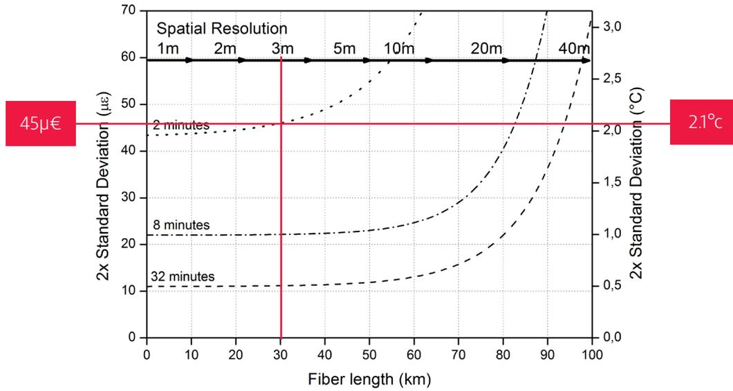
If you would like to measure 70km, using a short acquisition time 32 minutes: with 200ns pulse /20m spatial resolution will allow you to reach 70km with a measurement repeatability of  $15\mu\epsilon/0.75^{\circ}\text{C}$  (2 x the standard deviation).
