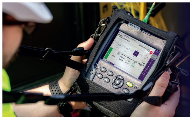
The lead engineer can view the user interface of a new tech's OTDR remotely from his office chair
