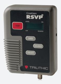
Of all available return path measurement systems, only the Guardian RSVP $^2$  tests C/(N+I) with the range needed to ensure trouble-free service. And it does it with a simple Pass/Fail test that can be performed in seconds.
